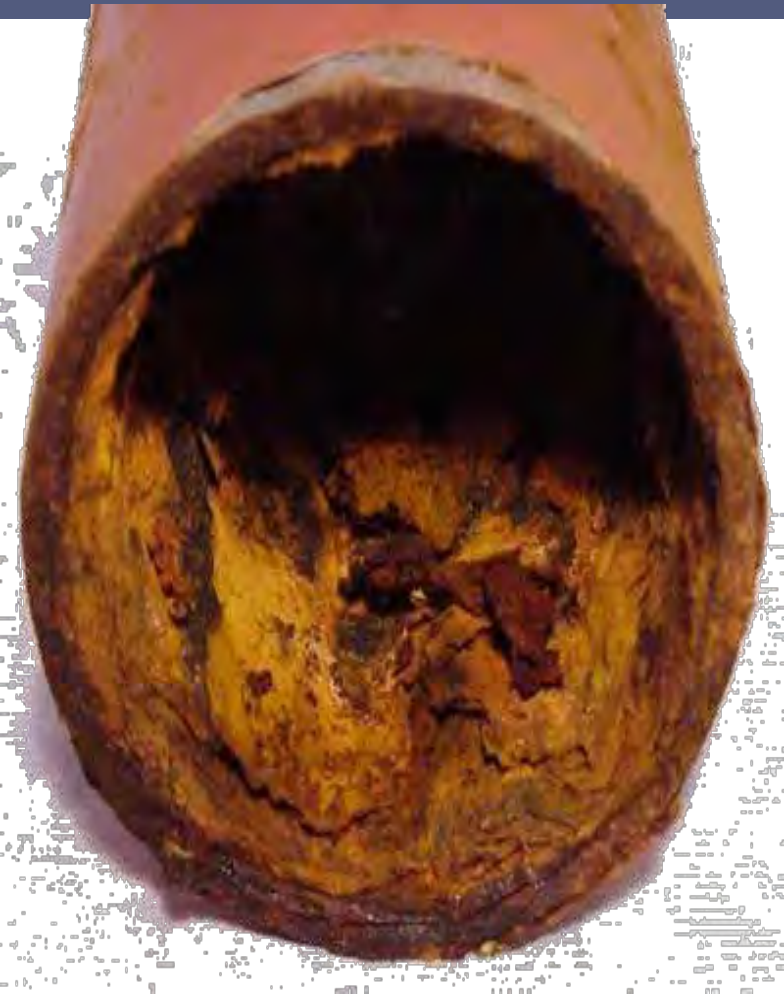
Rusted iron water pipe
